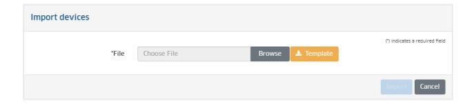
**3.** Click on the **Browse** button to locate the .csv file containing the APs, then click on the **Import** button at the bottom of the screen. The APs in the file will be imported into the Device Catalog.
